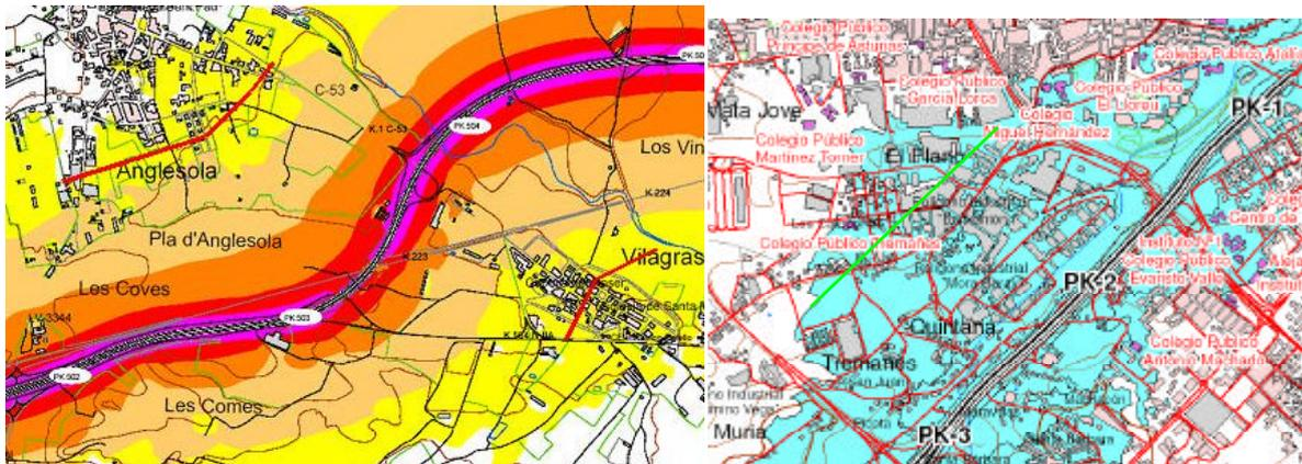
Figure 8: Noise Level Map and Noise Affection Map with a red and green line showing the validity limit distance of the calculation method.
