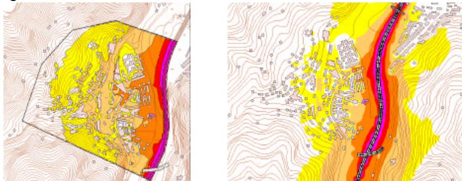
Figure 2: Strategic Noise Mapping applying Detailed methodology on the left and Basic methodology on the right.
